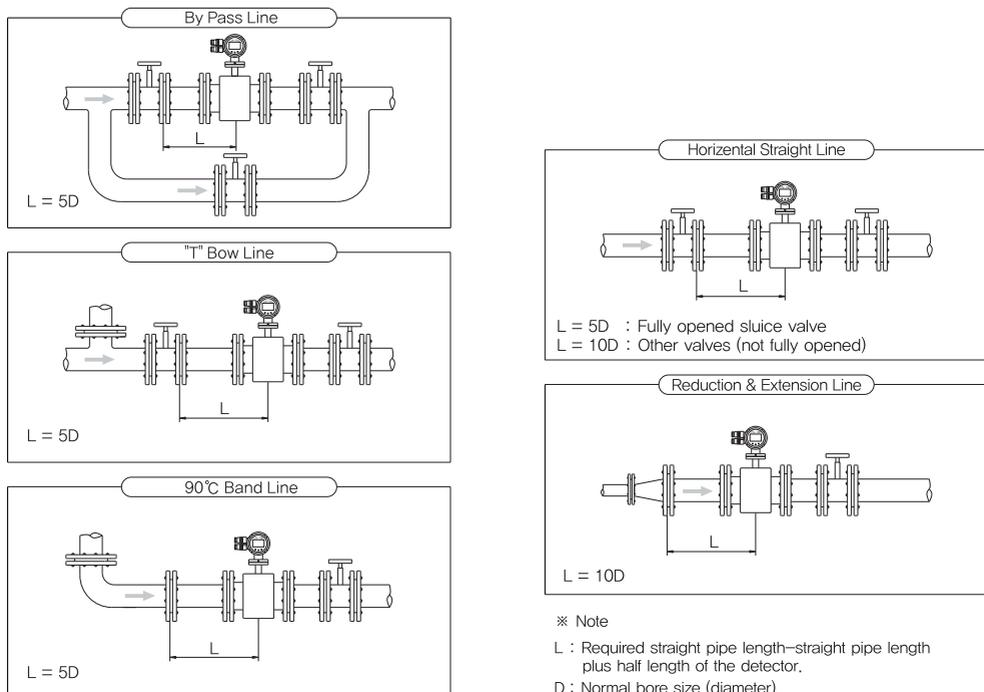
The figure above required straight pipe length on the upstream side
