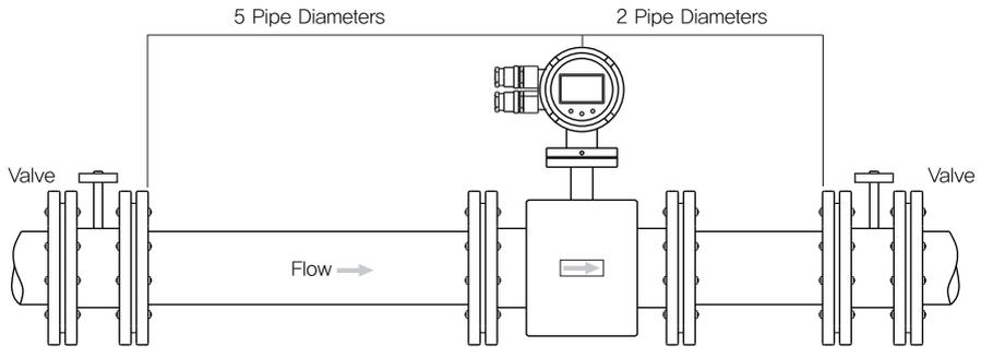
Upstream and Downstream straight pipe diameter
