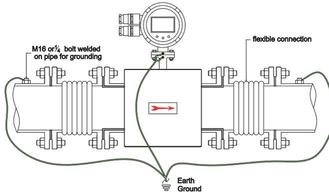
Figure 5. Ground for pipes with flexible connection
